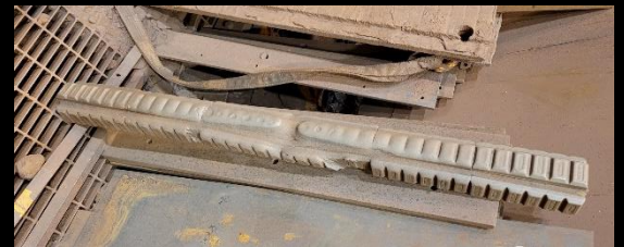
Old liner after one 20-week repair cycle
