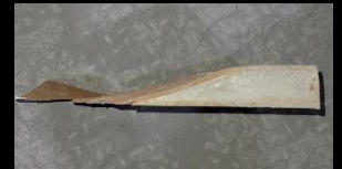
Ni-Hard liner after 3-months of run time
