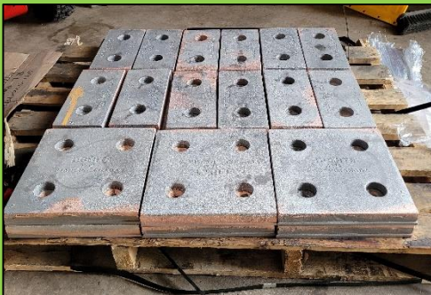
Domite 1.5"x12"x12" cast liners
