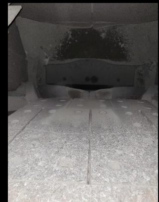
Domite liners after 6-months of run time
